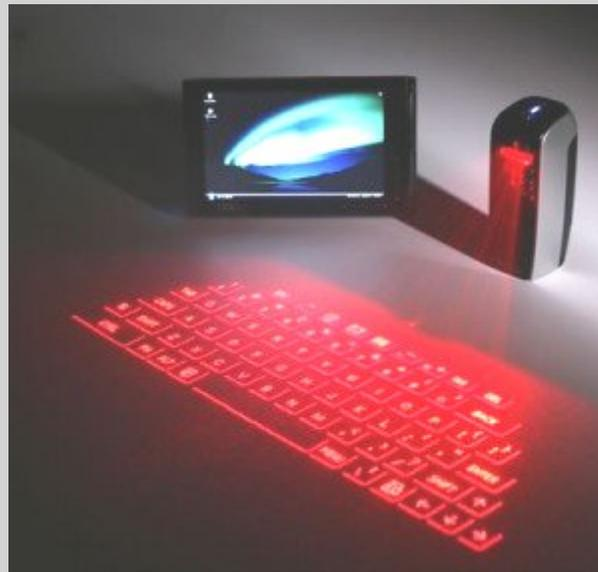
A virtual keyboard is a software and/or hardware component that allows a user to enter characters. A virtual keyboard can usually be operated with multiple input devices, which may include an actual keyboard, a computer mouse, a headmouse, and an eyemouse.
